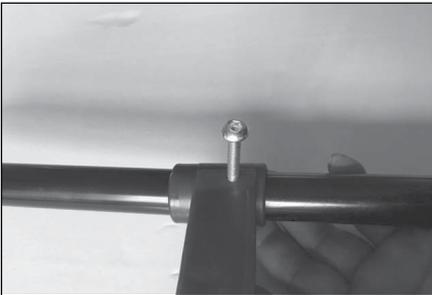
30. Return the ladder holding the nut and aims at using the Allen key (F) and repeat for each bindings.
