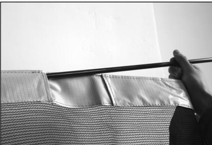
20. Inserting the sleeves (R) in the safety net (S) as follows. Be sure to let the end overtake the gap.
