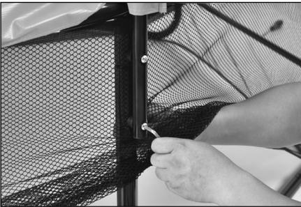
18. Finally with flange nuts (Q) and the keys (E and F), screw the amount on the flange with two fasteners. Repeat for the other poles.
