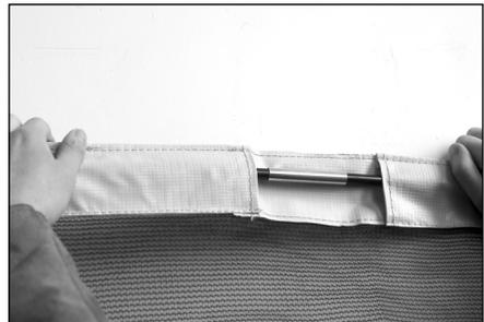
21. Insert the end of the sleeves (R) into the next one.
